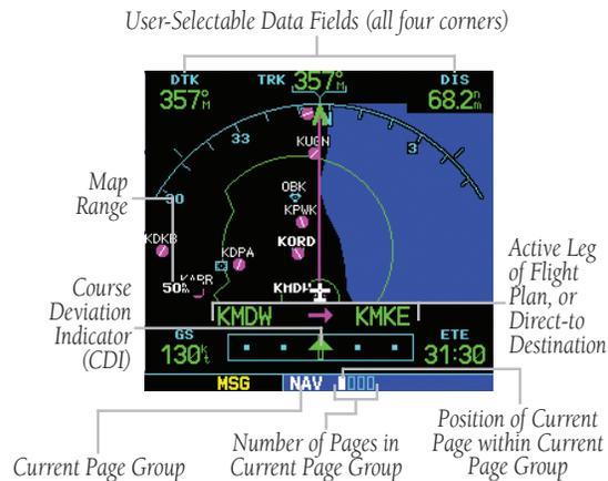
The following symbols are used on the Default NAV Page (directly above the CDI), to depict the 'active leg' of a flight plan or direct to:
