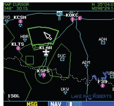
**Figure 3-15 Select Airspace with Target Pointer**
