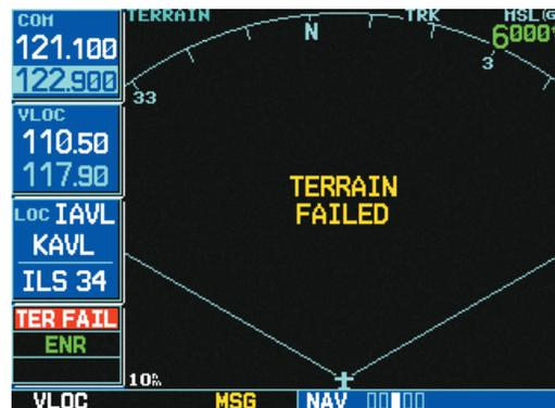
Figure 12-9: TERRAIN FAILED Display
