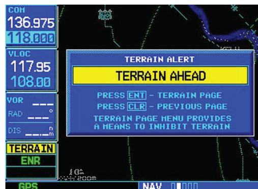
Figure 12-4 TERRAIN Caution Pop-up (Flashing)
