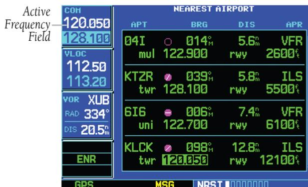
Figure 8-8 Frequency Moved to Active Field
