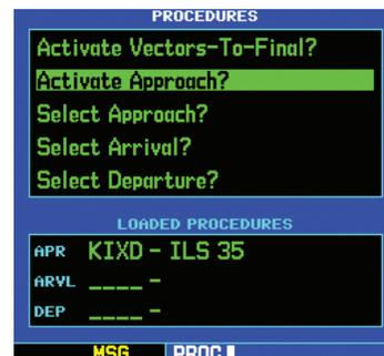
The 'Activate Vector-To-Final?' option allows the pilot to activate the final course segment of the approach. This option assumes the pilot will receive vectors to the FAF and provides guidance to intercept the final course, before reaching the FAF.
