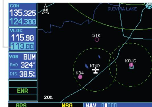
Figure 9-2 Tuning Cursor in VLOC Window
