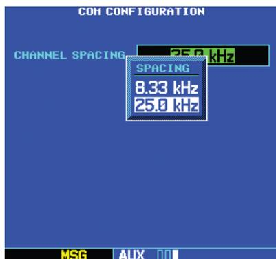
Figure 10-44 Channel Spacing Window
