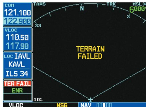
Figure 13-11: TAWS FAILED Display
