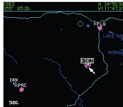
Figure 4-12 Panning Pointer Placed on Waypoint
