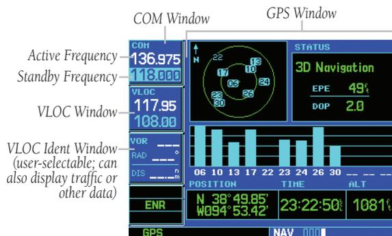
Each unique screen of information is referred to as a page. Pages are typically selected using the small and large **right** knobs, with the cursor removed from the GPS Window. See pages 6 and 7 for details on arrangement of the GNS 530's main pages.
