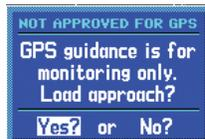
Not all approaches in the database are approved for GPS use. As the pilot selects an approach, a 'GPS' designation to the right of the procedure name indicates the procedure can be flown using the GPS receiver. Some procedures do not have this designation, meaning the GPS receiver may be used for supplemental navigation guidance only. ILS approaches, for example, must be flown by tuning the VLOC receiver to the proper frequency and coupling the VLOC receiver to the external CDI (or HSI).
