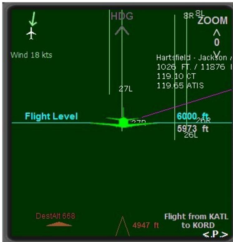
a. The position of the airplane shown in green at the center of the screen, when visible, indicates the relative distance from, and direction to, the intended flight level. It also shows the plane's relation to the intended track (magenta line). The peak of the terrain indicator will be moved up and down related to the elevation profile under the aircraft.
