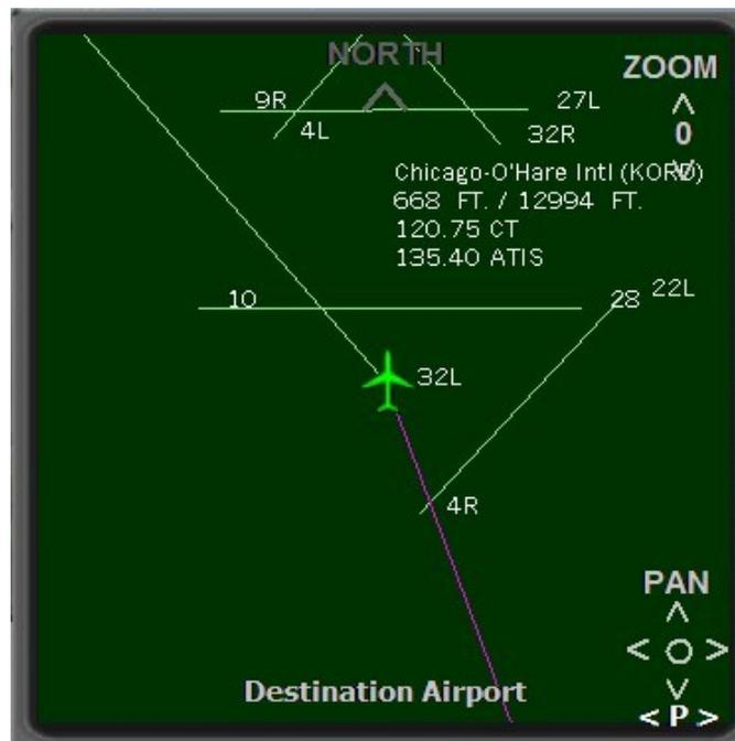
The magenta line displays the path of the current flight plan. All informations are self-explanatory.
